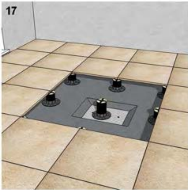
17 - For recesses, recessed manholes/drains or level changes, you may require longer NM pedestals which should be set out and installed in exactly the same manner as all other pedestals. See our full range of accessories so that you select the appropriate pedestals to suit your application.
