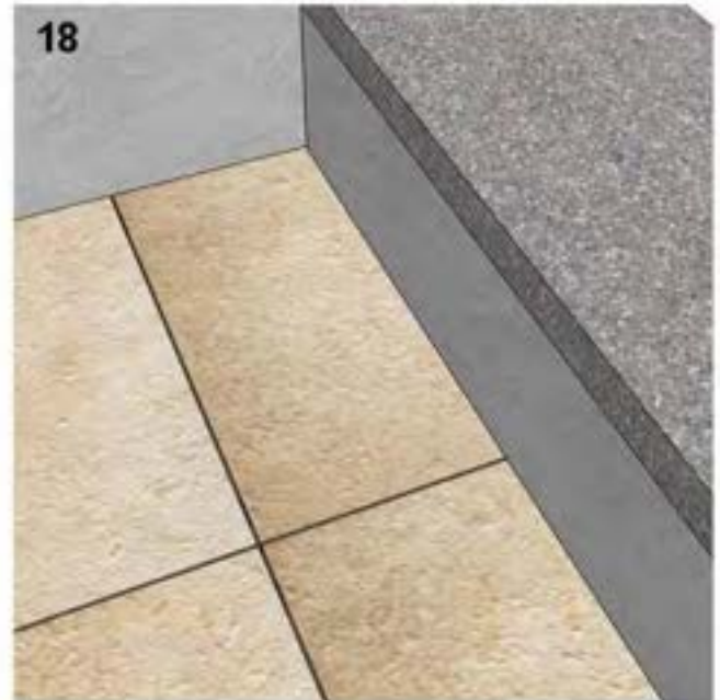
18 - Continue laying the pedestals and cut slabs in the same manner to all remaining edges requiring cut slabs.
