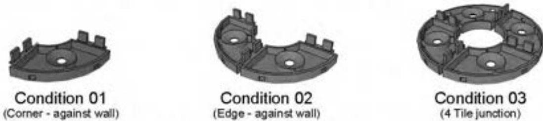
PAVING LAYING PATTERN AROUND A BUILDING INTERNAL CORNER.
