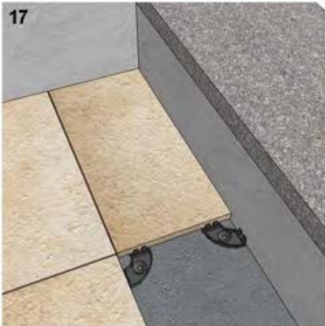
17 - Measure the distance to be paved between the last slab and the bounding wall or structure and subtract 6mm to determine the correct dimension of the cut slab and ensure a minimum 3mm gap between slabs and adjacent walls or structures. To cut the slabs we recommend you use a Rubi TC-180 circular saw with either dry blade (Rubi TCR31975) or wet blade (Rubi CPC230955).
