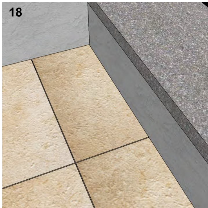
18 - Continue laying the pedestals and cut slabs in it the same manner to all remaining edges requiring cut slabs.
